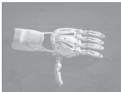
A 3D-printed prosthetic hand.
