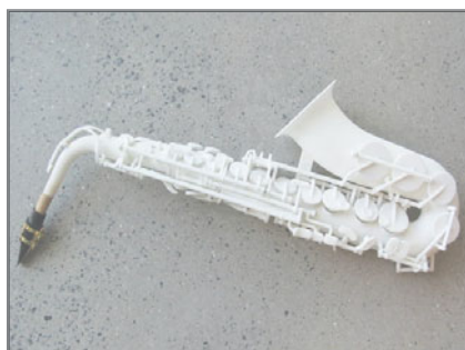
A working 3D-printed saxophone.
