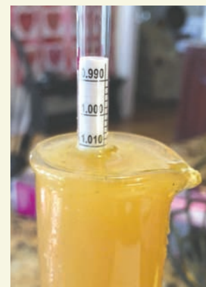
A gravity reading taken with a hydrometer on a sample of almost finished fermenting beer. All photos courtesy of Stephen Price
